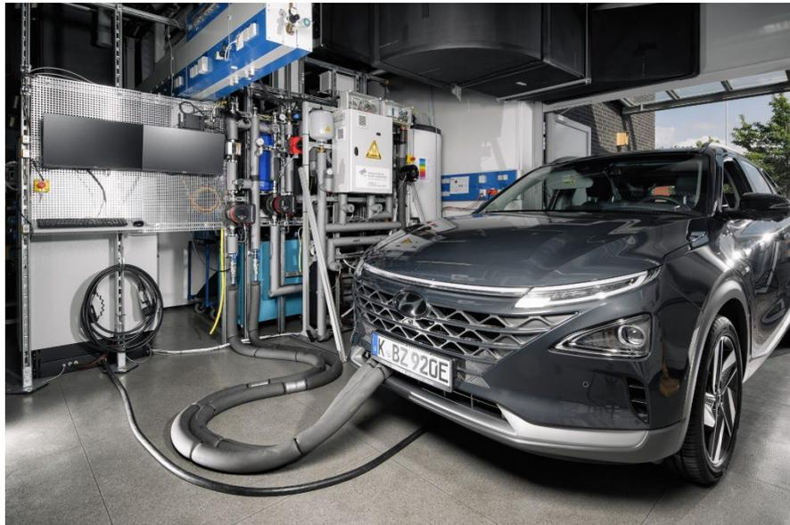
Figure 23. Test facility for the integration of fuel cell–electric vehicles into households. *Quelle: DLR*
