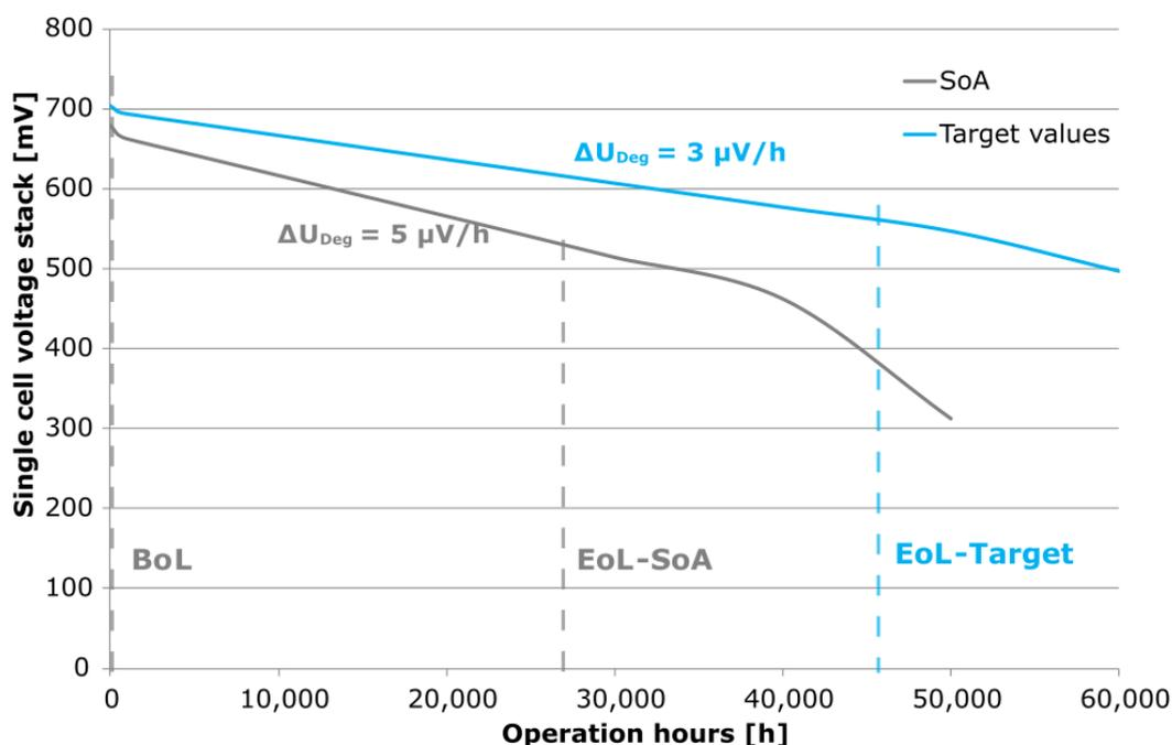
Figure 25. Examples of cell voltage curves from the Lifetime project.
