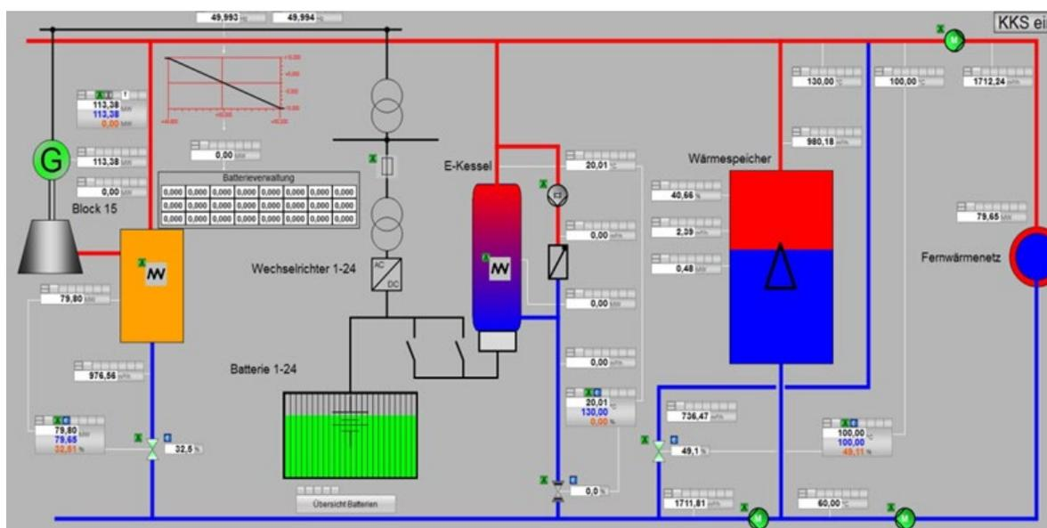
Figure 5. Functional operating diagram incorporating a battery, power-to-heat, and thermal energy storage.<sup>[20]</sup> Quelle: swb AG
