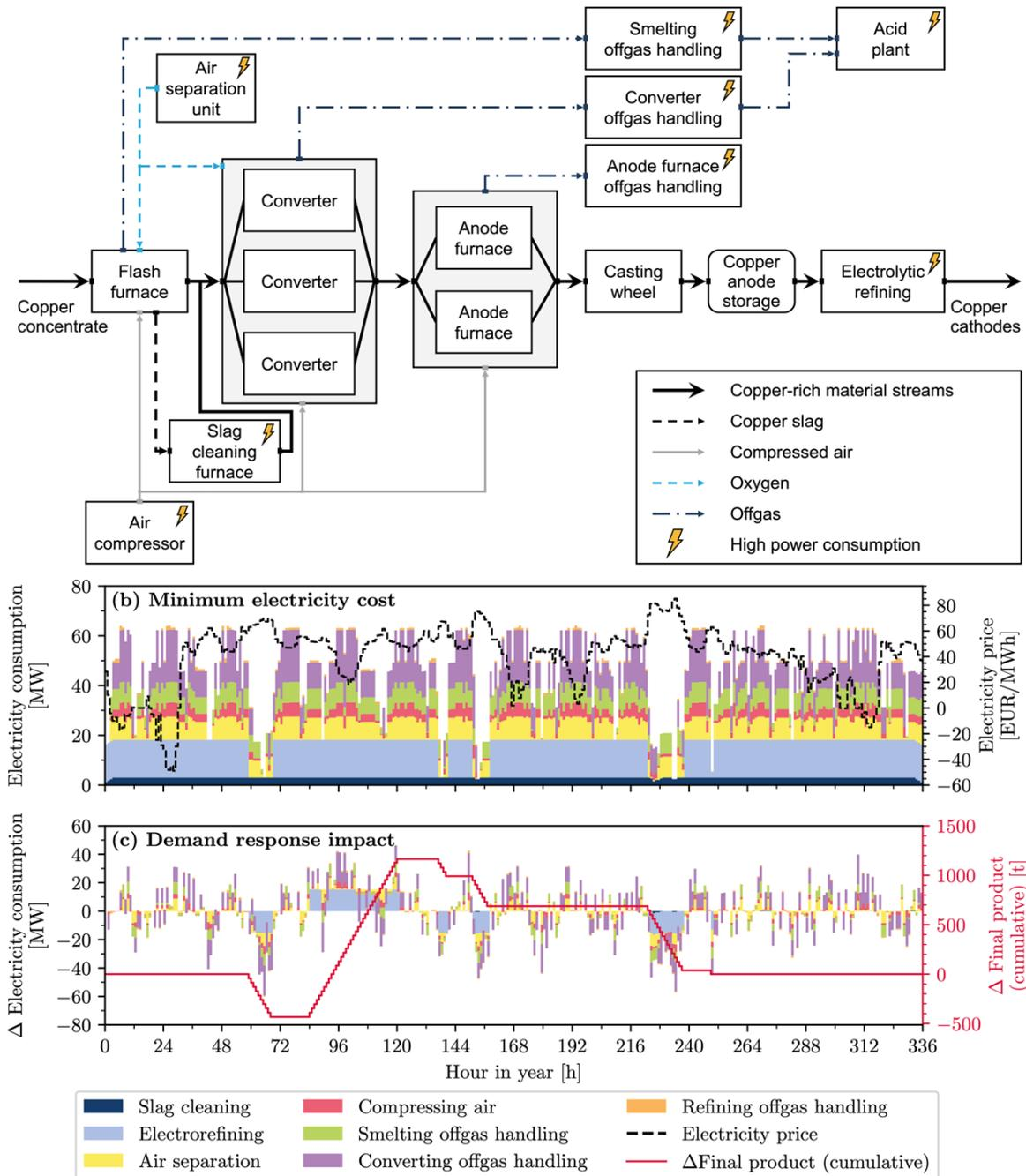
Figure 10. Demand response potential of copper production: Process flowsheet (top), optimal production schedule (center), and demand response impact (bottom) for the first two weeks of 2019. Left axis: electricity consumption; right axis: time-varying day-ahead prices (center) and cumulative change in the final product (bottom). The figure is adapted from Röben et al.<sup>[40]</sup>, [CC-BY-NC 4.0](https://creativecommons.org/licenses/by-nc/4.0/).
