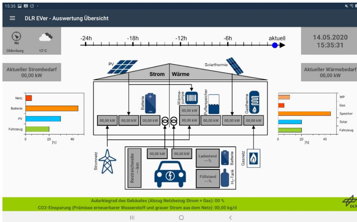
Figure 24. An app allows the power flows inside the complex “vehicle/building” system to be visually represented in real-time.
