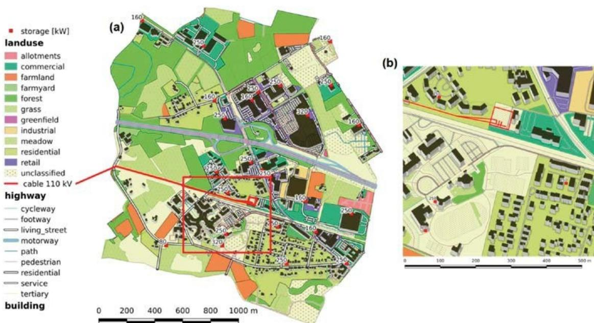
Figure 27. Cartographic representation of the urban energy infrastructure and potential locations for decentralized battery storage systems in a scenario for 2030 for the Wechloy district of Oldenburg (a). The enlarged area (b) shows the energy infrastructure and the distribution structures for battery storage systems.<sup>[96]</sup>
