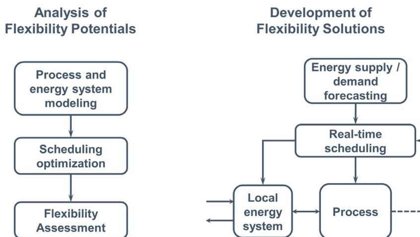
Figure 9. The FZJ and KIT use scheduling optimization to determine the flexibility potential of power-intensive production processes (left). Furthermore, they develop solutions for the real-time scheduling of flexible processes and their local energy supply systems (right).
