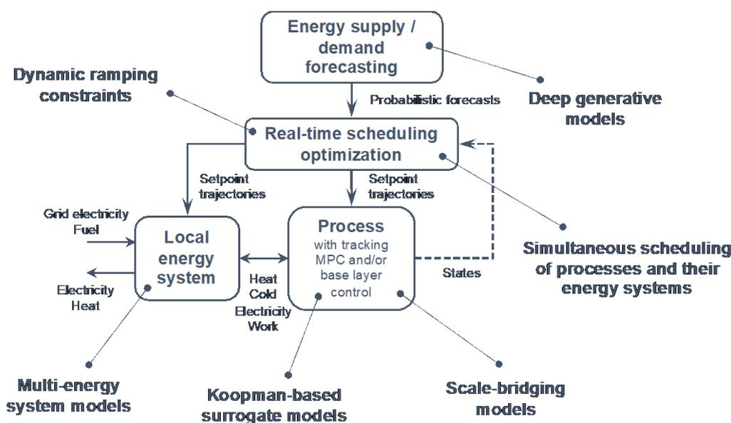
Figure 11. Flexibility solutions for the real-time scheduling of energy-intensive industrial processes and their local energy supply systems developed by the FZJ and KIT.
