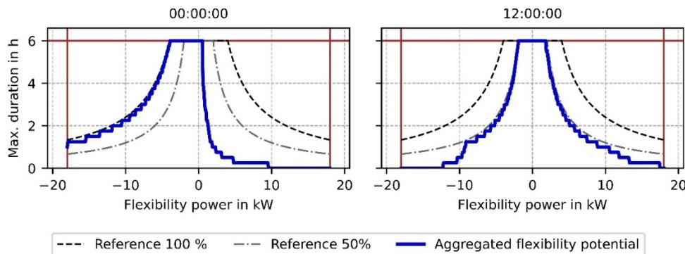
Figure 16. Aggregated flexibility potential.<sup>[64]</sup>
