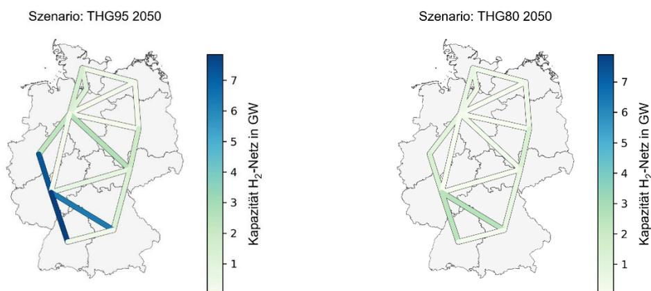
Figure 3. Expansion of the domestic German hydrogen transport network in the two scenarios (THG95/THG80) investigated in the MuSeKo project for the year 2050.
