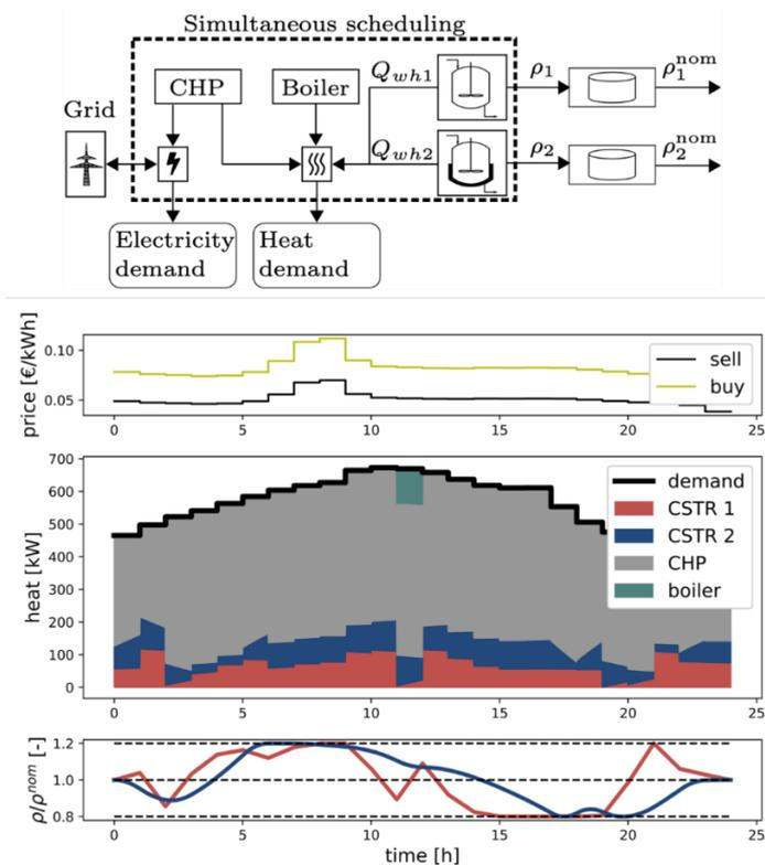
Figure 13. Dynamic ramping constraints (DRCs) for the simultaneous scheduling of two CSTRs and a multi-energy system consisting of a combined heat and power plant (CHP) and an electric boiler: The production  $\rho$  is shifted in time such that the boiler must rarely be turned on, as CSTR waste heat is used to partially cover the on-site heat demand. The figure is adapted from Baader et al.<sup>[54]</sup>, copyright: Elsevier.
