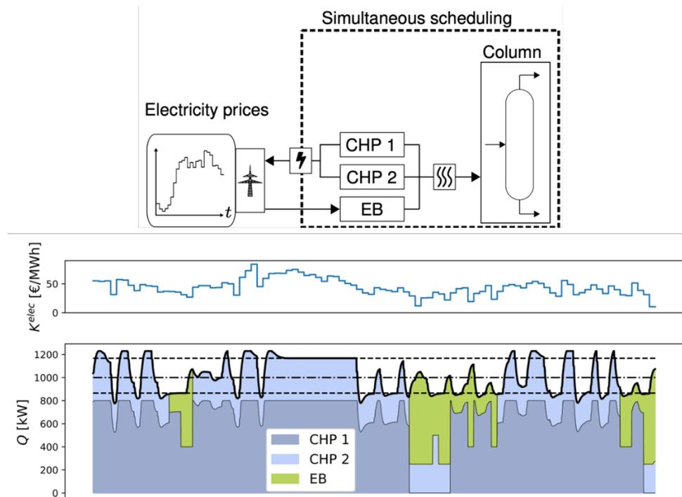
Figure 12. Simultaneous dynamic scheduling (SDS) of a distillation column and its local energy supply system consisting of two combined heat and power plants (CHP1 and CHP2) and an electric boiler (EB): In times of low electricity prices  $K^{elec}$ , the electric boiler is used to supply parts of the heating duty  $Q$ . The figure is adapted from Baader et al.<sup>[50]</sup>, [CC-BY 4.0](https://creativecommons.org/licenses/by/4.0/).
