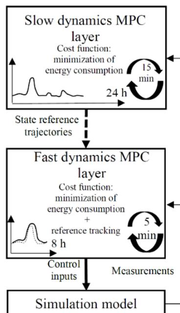
Figure 19. Structure of the hierarchical MPC concept.<sup>[80]</sup>
