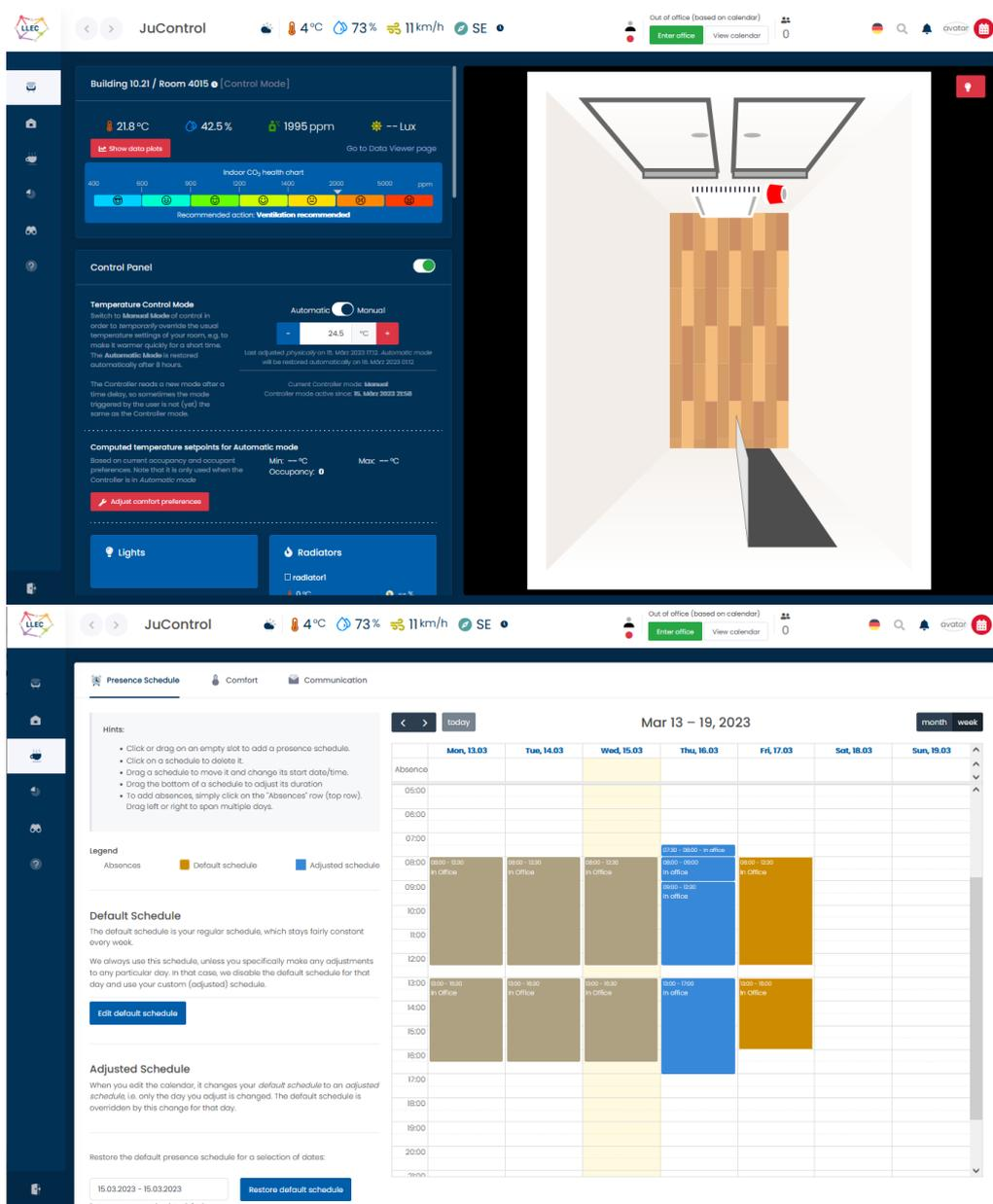
Figure 21. Screenshot showing the main page in JuControl, displaying measurement data and the control interface for a typical office (top); screenshot of a “presence calendar,” showing the anticipated presence in the office of a typical user (bottom).<sup>[74]</sup>
