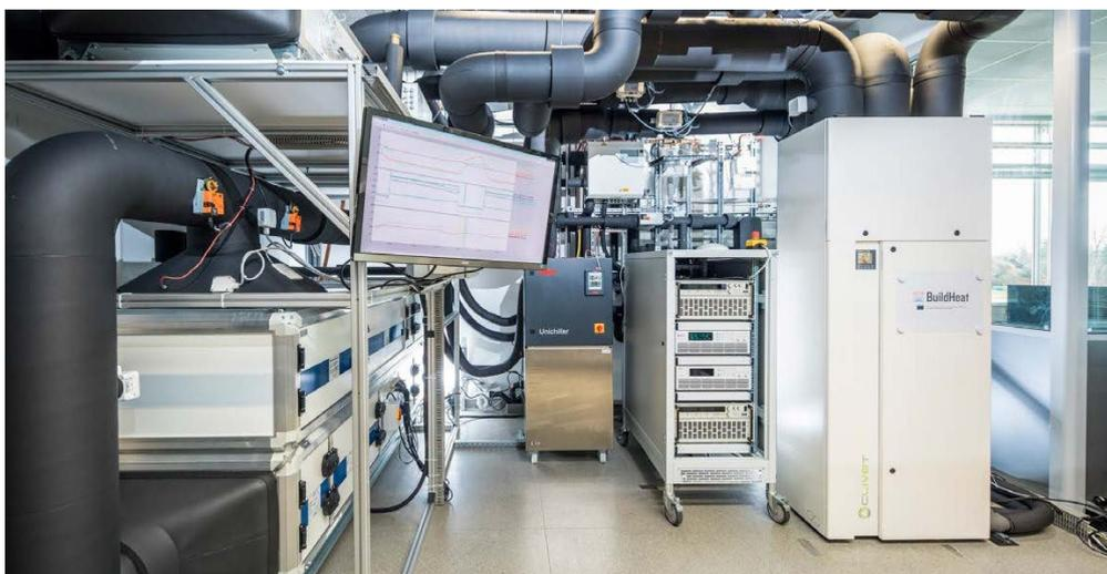
*Figure 17. Test bench facility for evaluating the air-to-air heat pump system at the DLR. Quelle: DLR*
