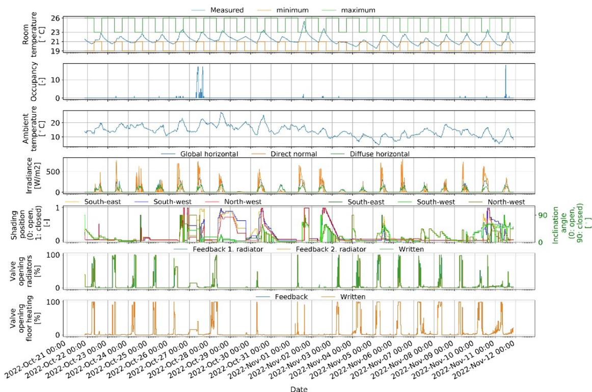
Figure 20. Typical MPC results from the first real-world application of the JModelica-based MPC framework (from October 11 to November 7, 2022).<sup>[70]</sup>
