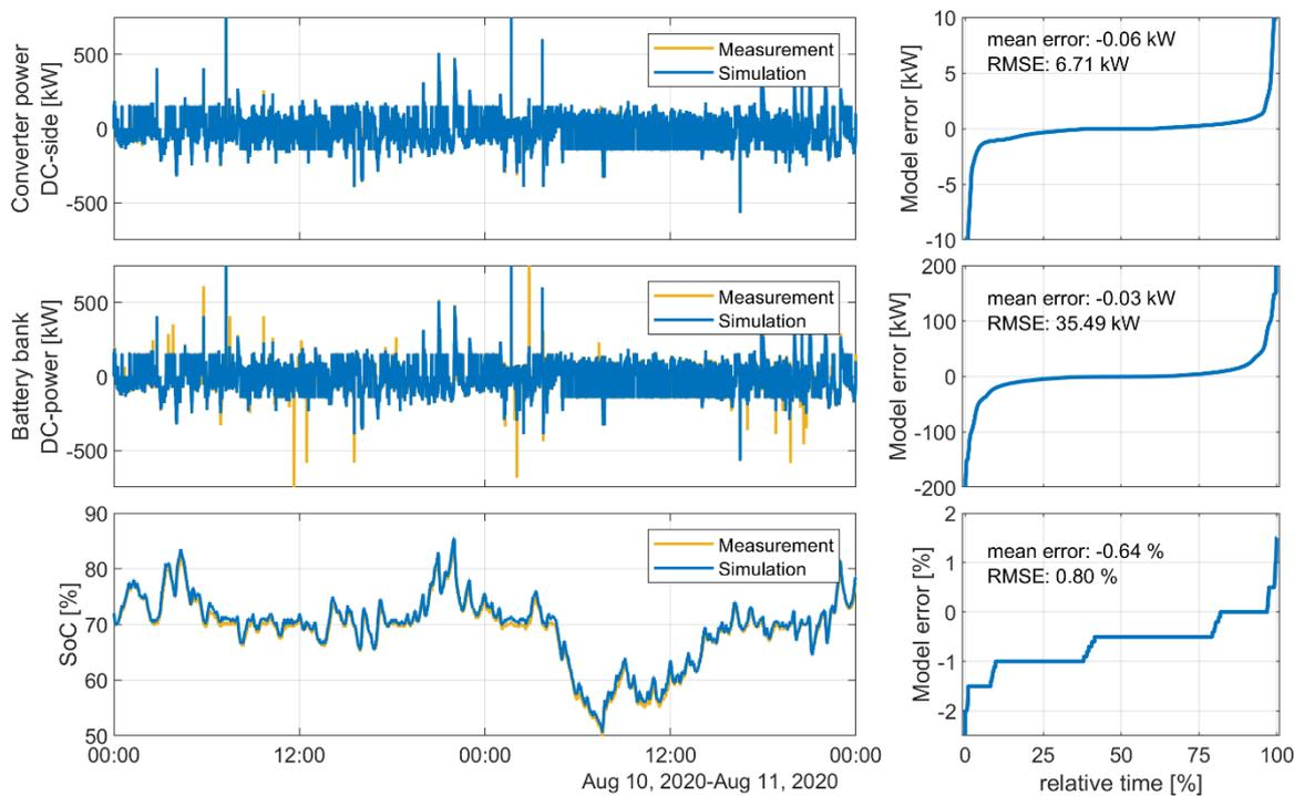
Figure 7. Simulation of one operating day.<sup>[25]</sup>
