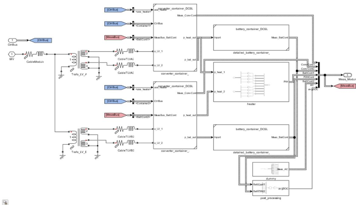
Figure 6. HyReK module as a detailed electrical model (sub-part of the overall system).<sup>[20]</sup>
