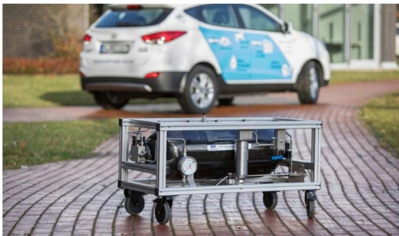
Figure 2. DLR's refueling module consisting of a type 4 hydrogen tank that is used in research projects to determine the hydrogen quality at refueling stations. Quelle: DLR
