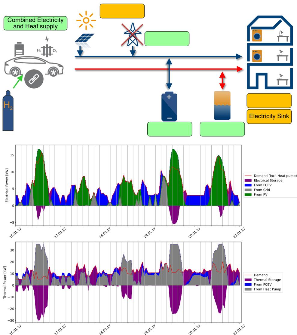
Figure 22. Graphic representation of the “oemof” optimization model used, which connects a building and vehicle via an energy interface (top). Calculation in oemof for feeding electrical energy from a parked fuel cell car back into a single-family home.<sup>[87]</sup>
