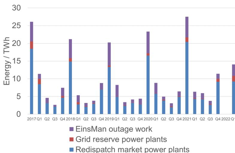
Figure 1. Network congestion management measures for the years 2017–2022 (adapted from Bundesnetzagentur).<sup>[7]</sup>
